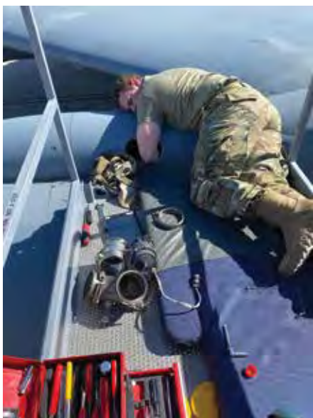
Staff Sgt. Cody Moss changes a bleed-air shutoff valve at the Utah Air National Guard. Members of the UTANG board aircraft 0275 departing to Joint Base Andrews prior to the 59th Presidential Inauguration. Members of the fuels shop pose for a photo while preparing for departure to Al Udeid Air Base, Qatar. Staff Sgt. Ted Hess cleaning an engine exhaust gas temperature canon plug. The picture was taken during a 24-month ISO inspection in February of 2021.
