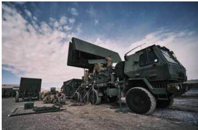
Master Sgt. Steven Smellie, Staff Sgt. Joshua Johnson and Senior Airman Alexander Kondo, members of the 109th Air Control Squadron work at unfolding the AN/TPS-75 Radar at Wendover, Nevada, March 2021.
