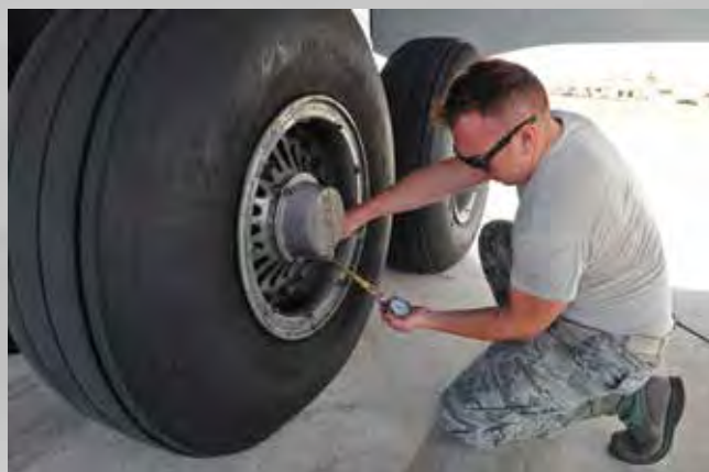
Master Sgt. George LaCome, 151st Maintenance Group crew chief, checks the tire pressure on a KC-135R during a preflight inspection at Andersen Air Force Base, Guam, prior to the six-person crews aeromedical-evacuation mission in the Pacific theater from Feb. 8-25, 2017.
