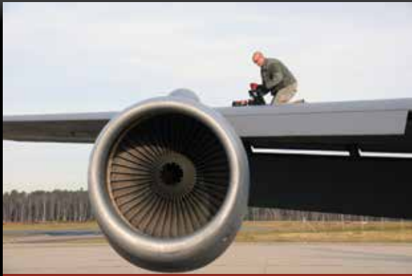
During training in Germany, Senior Airman Josh Wasden, a crew chief with the 151st Maintenance Group, adds hydraulic fluid to a KC-135 Stratotanker on Jan. 6, 2015.
