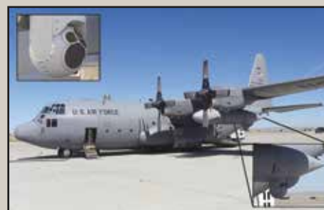
Upload of Senior Scout shelter. Pod-mounted installation of EO/IR sensor.
