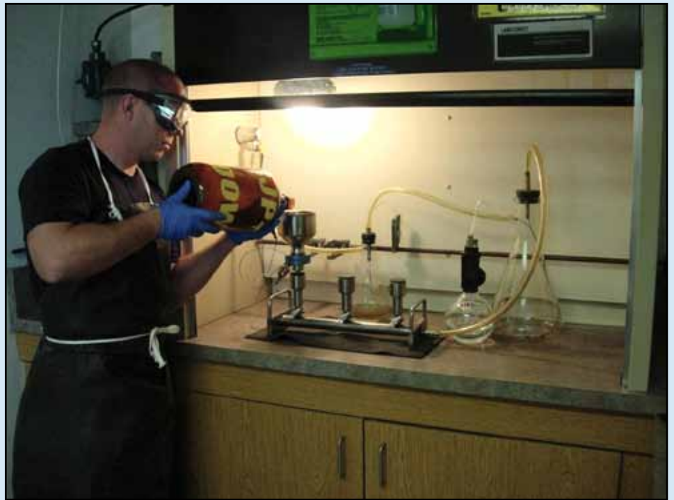
Staff Sergeant John Stroh performs a filtration test on JP8 jet fuel.
